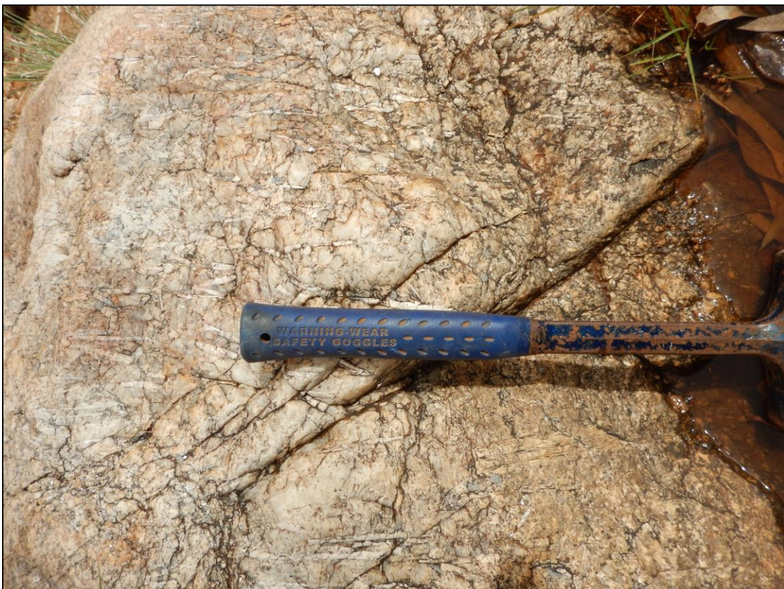
Figure 4: Kathleen Valley Project – Mt Mann pegmatite/close up showing large white spodumene crystals (Sample 160614_14A).
