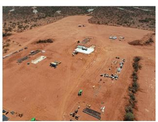
Figure 4: Fine ore bin foundation pouring commenced
