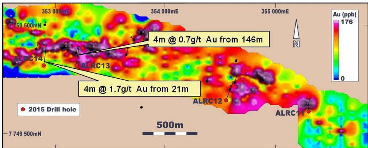
Figure 2: Allandale prospect - Drill hole plan on gold-in-soil image showing better gold intersections.
